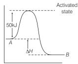
$$\begin{array}{ll} \therefore & \Delta H \ (B \rightarrow A) = 10 \ \text{kJ/mol} \\ E_{\text{a}} \ \ (A \rightarrow \text{activated state}) = 50 \ \text{kJ/mol} \\ \therefore & E_{\text{a}} \ \ (B \rightarrow \text{activated state}) = 50 + 10 = 60 \ \ \text{kJ/mol} \\ \end{array}$$
